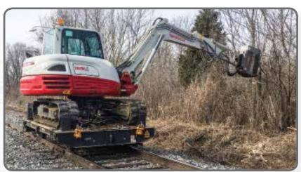
Dymax Rail Rider MP8 at work in Missouri on Kansas City Southern lines. Drum style brushcutters on small excavators are a productive tool.
