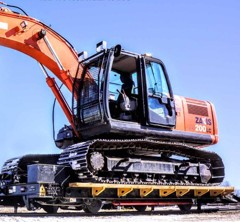
RAIL RIDER MPX - THE MOST ADVANCED MOTORIZED CART FOR TRACKED EXCAVATORS
