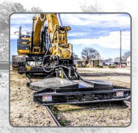
Dymax Rail Rider MP1620 with VortexMax ready to demolish brush and vegetation alongside rail line in Kansas.
