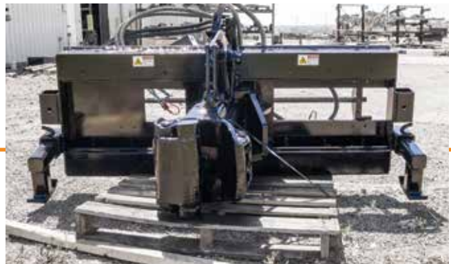
Tractor - 3 point hitch with hydraulic positioner
